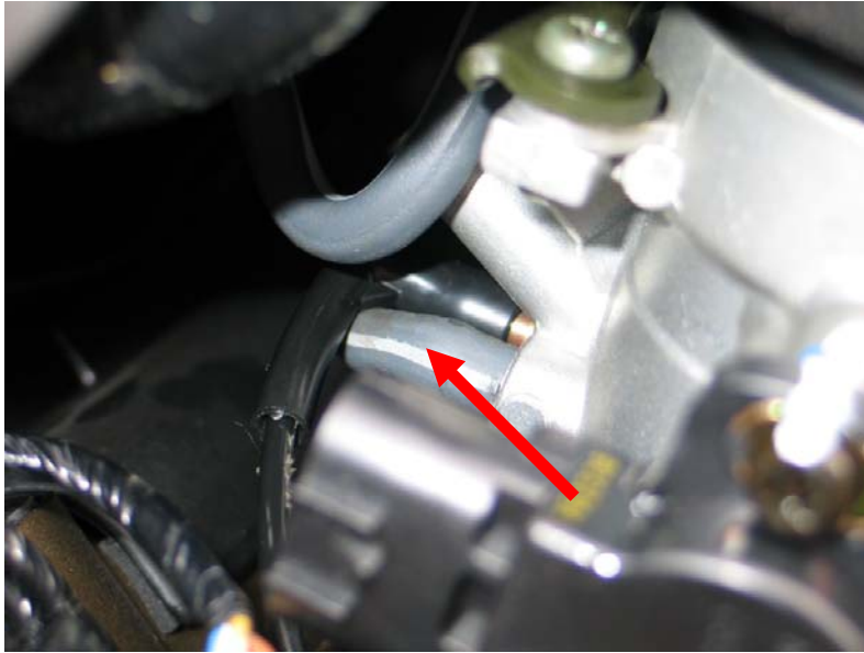
Detail of damper elbow fitted to stub on throttle body.
